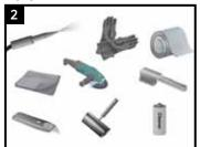
Appropriate tools for surface abrasion (wire brush, grit blaster); Standard safety equipment; gloves, goggles, hard hat, etc; Power wire brush, grinder, abrasive paper; Knife, rags
