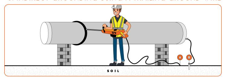
Indirect grounding using a trailing ground. This grounding alternative allows holiday testing without an obstructing cable, if direct grounding is not possible.
