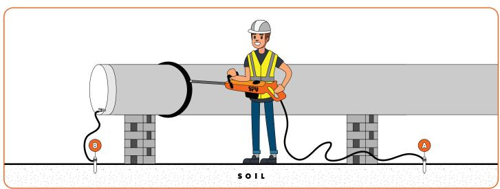
An additional grounding rod allows the direct grounding of the holiday detector, if the bare pipe end (cut back) cannot be connected using the standard 25 ft ground cable. If desired SPY® also makes custom length ground cables of any length, contact sales for details.
