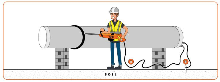
Direct grounding using the standard 25 ft ground cable is the most reliable form of grounding which offers a direct connection between the holiday detector and the non-insulated pipe end (cut back) to be tested.
