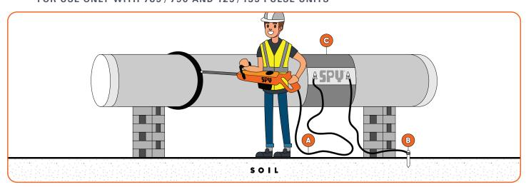
The grounding collar is used if no direct or indirect grounding is possible. The grounding collar is also recommended in case of bad conducting or extremely dry soil. Refer to the Appendix on page 4 for more details.
