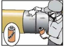
3. Insure that surfaces are clean of grease, oil, salts and other contaminants. If necessary, use Acetone, MEK or other suitable solvent. Perform cleaning when pipe is 3°C (5°F) above dew point.
