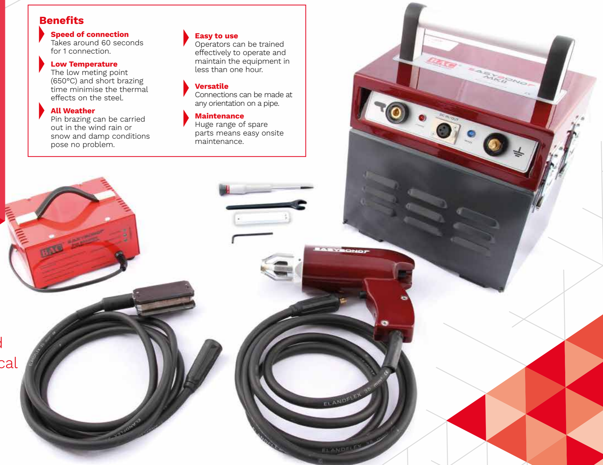
1. Clean to a bright metal 2. Load gun with pin & ferrule 3. Adjust as required 4. Pin Braze 5. Test the connection
