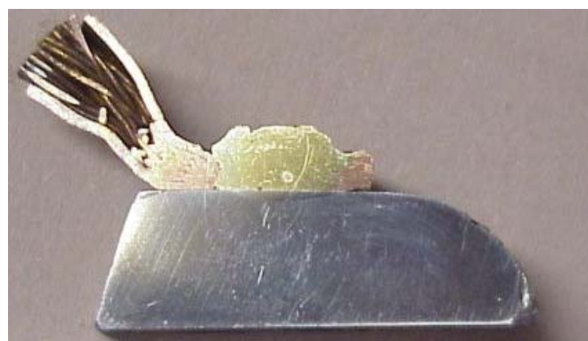
Cross section of 8mm brazing pin and integrated Bond.
