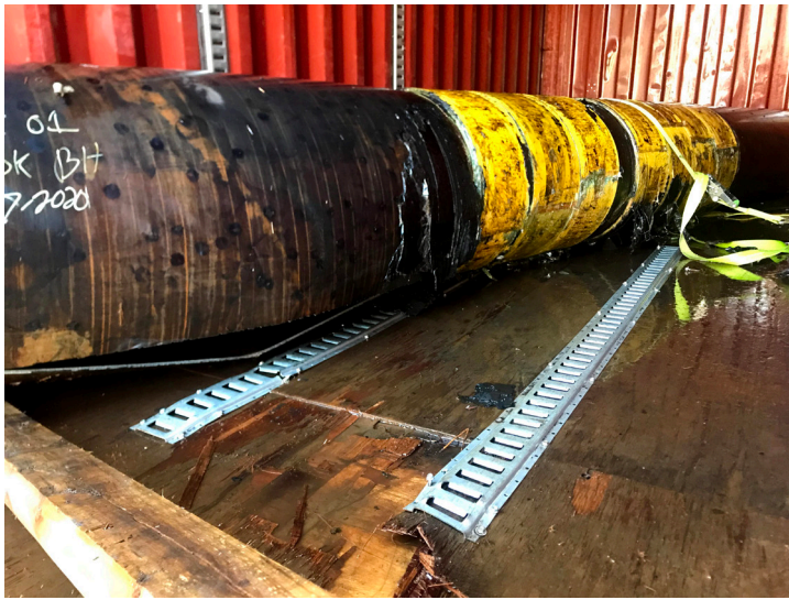
Figure 1. The testing programme for the 25-year old Clock Spring® repair was designed to gradually increase pressure to 1455 psi (100.3 bar), which is 1.5 times the MAOP of the pipeline, where the MAOP was 970 psi (66.9 bar). The composite repair showed no damage when the repaired pipeline section was pressurised to the target value of 1455 psi (100.3 bar) and held at that pressure for five minutes. (Photo courtesy of CSNRI).
