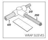
**ANSWER 1a:** You can often shim one or two cable sizes to fit a larger mold. Use a wrap sleeve, CADWELD Part No. **B140A.** Wrap the shim around each cable to build it up to a 4/0 size. Then use the 4/0 molds to make the connection. We recommend that you keep a package of wrap sleeves handy.
