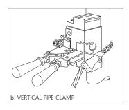
b. If welding to a vertical pipe, the CADWELD Pipe Clamp works well. It is a single unit incorporating both the pipe clamp and the handle clamp. Part numbers for the different mold sizes and applications are as follows:
