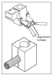
ANSWER 11a: The first thing to check is the adjustment of the handles, especially if the handles are new. Just in front of the grips is the adjustment linkage. Remove the key and pin. Turn the linkage counterclockwise to tighten the locking action and clockwise to loosen the locking action. Test the locking action and then replace the pin and key.
