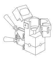
QUESTION 30: I've noticed in your catalog a separate listing for "Heavy Duty" CADWELD Connections. Why Heavy Duty? **ANSWER:** Heavy Duty Connections are often used for making connections to aged cable during grounding system expansion projects (for example, expanding the site of a substation grounding grid). When field conditions are unusually bad, CADWELD Heavy Duty connections provide a solution.
