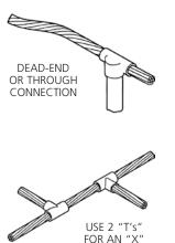
**ANSWER 3c:** For ground rods, use **Type GT** through cable connections. When the cable dead-ends at the ground rod, just let it extend past the rod 2" (through the mold) when making the connection.
