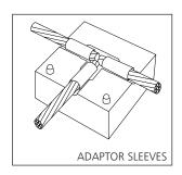
**ANSWER 1b:** Use an adaptor sleeve which is sized for specific cables to build up 2/0 to fit the 4/0 mold. Select sleeve Part No. **B1332Q** for this example. Adaptor sleeves cost more but they take less time.
