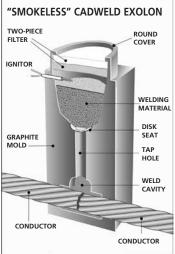
**ANSWER:** To deal with such situations, Pentair developed the CADWELD EXOLON low-emission welding process. The CADWELD EXOLON system produces the same permanent, highly reliable welded bonds as the standard CADWELD process, but without the smoke usually associated with the exothermic welding process.
