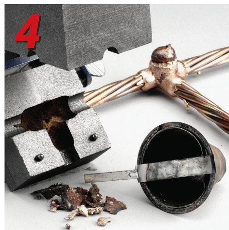
Open the mold and remove the expended steel cup – no special disposal required
