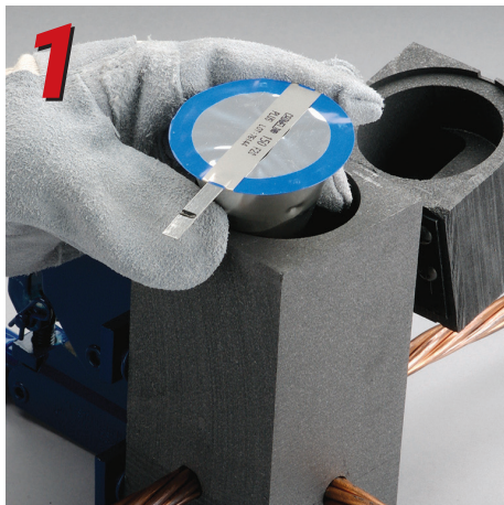
Insert Cadweld Plus cup into mold (may require use of a cover/baffle)
