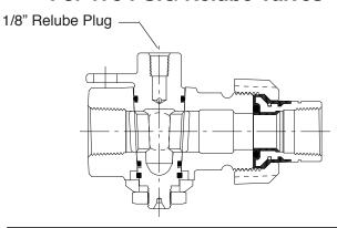
NOTE: These valves are designed for use with natural, manufactured or LP gas only.
