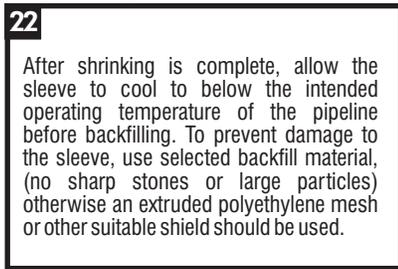
After shrinking is complete, allow the sleeve to cool to below the intended operating temperature of the pipeline before backfilling. To prevent damage to the sleeve, use selected backfill material, (no sharp stones or large particles) otherwise an extruded polyethylene mesh or other suitable shield should be used.
