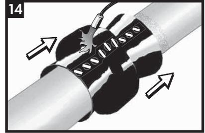
Continue heating from the centre towards the pipe on each side so that the sleeve begins to recover on one side then the other. If the sleeve begins to fan outwards, use a gloved hand to guide the recovery towards the pipe.
