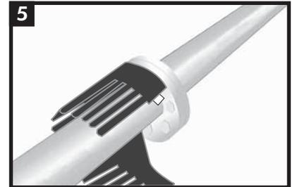
Wrap the finger skirting around one half of the flange. The fingers should point towards the flange bolts.
