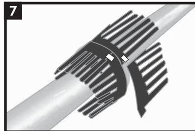
Centre the protective skirting over the flange. Using the tape provide, attach the skirting to the flange. Begin wrapping the protective skirting around flange tightly.
