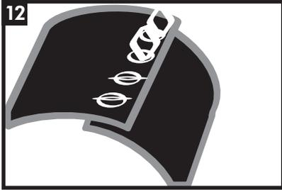
Insert the clips through the holes, push down the closure area to conform to the joint profile. Insert the flat-head screwdriver into the clips and flatten clips with gentle blows from a hammer (use needle-nose pliers if clips become bent or irregularly shaped).
