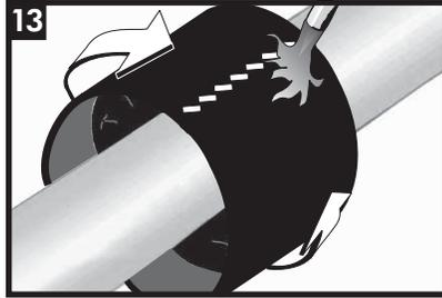
Using broad strokes, heat the sleeve circumferentially around the pipe starting with the centre of the flange. Do not touch or damage the sleeve while it is hot.
