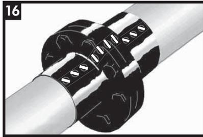
Gently push down the sleeve so it conforms to the flange profile.
