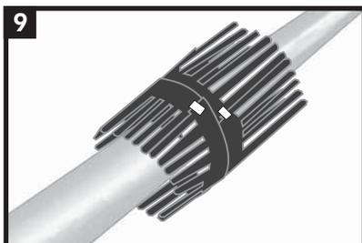
Ensure the skirting is well secured to the flange and it will protect the sleeve from the flange bolts.
