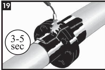
Apply low heat to the closure and press it down with a gloved hand until it conforms to the flange profile.
