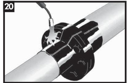
Apply an even final heating to the entire closure seal.
