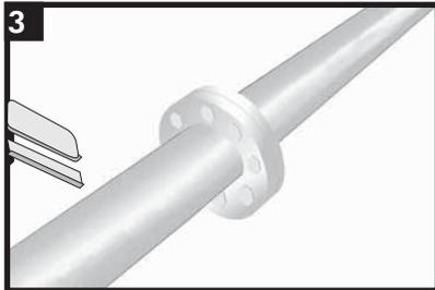
Remove all dirt and rust by grit or shot blasting, needle gunning and wire brushing, or other approved technique.
