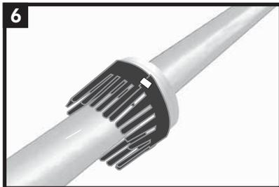
Finish wrapping the skirting around the flange. Use a piece of tape to secure the skirting in place.
