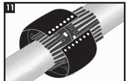
Centre the two middle clips on either side of the flange and wrap the sleeve around the joint to match the insert holes over the clips.
