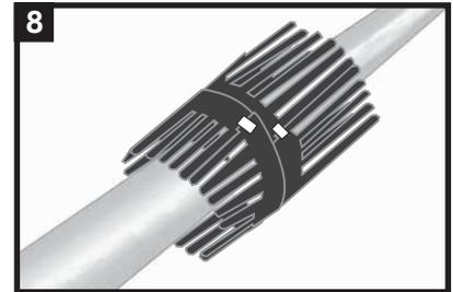
Finish wrapping the protective skirting around the flange. Using the supplied tape, firmly attached the protective skirting around the flange.
