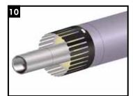
Finish wrapping the profile support skirting around the casing pipe. Use the supplied tape to firmly attach it to the casing pipe.
