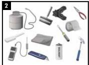
Propane tank, hose, torch & regulator. Appropriate tools for surface abrasion. Knife, roller, rags & approved solvent cleanser. Temperature measuring device. Hammer, small flat-head screw driver, needle-nose pliers. Standard safety equipment; gloves, goggles, hard hat, att
