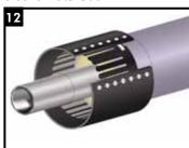
Centre the two middle clips on the edge of the casing pipe and wrap the sleeve around the joint to match the insert holes over the clips.
