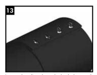
Insert the clips through the holes, push down the closure area to conform to the joint profile. Insert the flat-head screwdriver into the clips and flatten clips with gentle blows from a hammer (use needle-nose pliers if clips become bent or irregularly shaped).
