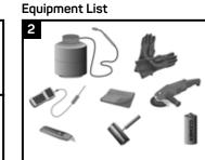
Propane tank, hose, torch & regulator; Appropriate tools for surface abrasion and cleaning (60-80 grit sand paper and a power wire or hand wire brush); Knife, roller, clean white rags & approved cleaner; Digital thermometer with suitable probe; Standard safety equipment; gloves, goggles, hard hat, ote
