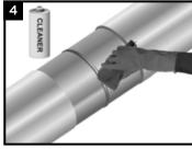
Clean exposed steel and adjacent pipe coating with an approved cleaner and a clean white rag to remove the presence of oil, grease, and other contaminants.
