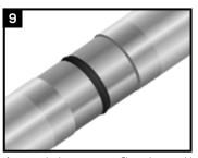
If required, changes in profile at butt-weld straps and bell & spigot details can be filled with an approved filler tape sealant prior to sleeve application.
