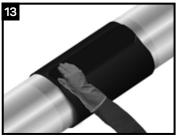
Remove any release liners from the closure. Centre the closure on the overlapping sleeve. Press down firmly
