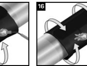
one end of the sleeve until recovery is complete. In a similar manner, heat and shrink
