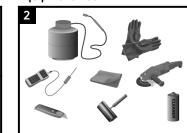
Propane tank, hose, torch & regulator; Appropriate tools for surface abrasion and cleaning (60-80 grit sand paper and a power wire or hand wire brush); Knife, roller, clean white rags & approved cleaner; Digital thermometer with suitable probe; Standard safety equipment; gloves, goggles, hard hat, etc.
