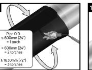
Using the appropriate sized torch, begin at the centre of the sleeve and heat circumferentially around the pipe. Use broad strokes. If utilizing two torches, operators should work on opposite sides of pipe.
