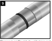
Changes in profile at butt-weld straps and bell & spigot details (when step down is  $\geq 1/4''$ ) are to be filled with the approved filler tape sealant prior to sleeve application.
