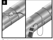
Pre-heat the joint area using propane torches to 105-140°F. The bare steel area should be heated to 140°F. If the pipe is Polyurethane coated, it should be heated to 140°F as well. If the pipe is tape coated, do not heat the tape coating to more than 110°F or damage may occur. In cold or windy conditions, the preheat temperatures for steel and Polyurethane may be increased to 160°F.
