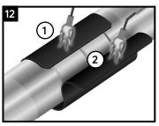
Wrap the sleeve loosely around the pipe, ensuring the appropriate overlap. Gently heat the backing of the underlap and the adhesive side of the overlap. Press the overlap into place.
