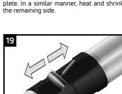
Continue the procedure by also firmly rolling the closure with long horizontal strokes
