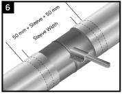
Ensure that the pipe is dry before cleaning. The bare steel joint area must be cleaned to a minimum of St2, wire brush finish. Remove all loose rust, mill scale, loose coating, etc. Lightly abrade the pipe coating adjacent to the weld area with 60-80 grit sand paper, to a distance of 50mm (2") beyond each end of the sleeve width.
