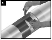
Apply mixed epoxy to a uniform specified thickness of 4-6 mils (100-150 microns) on all exposed bare metal using the applicator pads as supplied or an approved tool. Do not apply the epoxy to the mainline coating.
