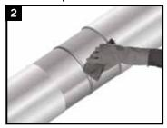
Clean exposed steel and adjacent pipe coating according to SSPC SP 1 to remove the presence of oil, grease, and other contaminants. Ensure that the pipe is at least 3°C (5°F) above the dew point before cleaning.
