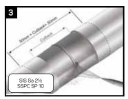
Thoroughly clean the cutback area to "near white metal" SIS Sa 2½ (SSPC-SP10) or equivalent. Materials used for abrasive blasting shall produce an angular surface profile of 2.5-5 mils (64-127 µm) Lightly abrade at least 50mm (2") of the line coating on each side of cutback area.
