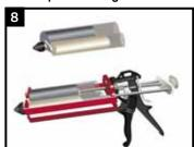
Canusa's HBE is available in a 2-component cartridge. Typical use is as a holiday repair coating on FBE coated pipe or for recently coated rehabilitation projects using HBE-95 or HBE-HT products. The cartridge fits into a universal 2-component cartridge dispenser that is available from Canusa.
