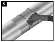
Wipe clean or air blast the steel and coated areas to remove foreign materials.
