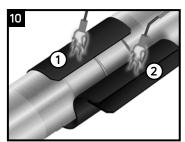
Wrap the sleeve loosely around the pipe, ensuring the appropriate overlap. Gently heat the backing of the underlap and the adhesive side of the overlap.
