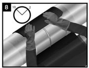
Centre the sleeve over the joint so that the sleeve overlaps between the 10 and 2 o'clock positions. Press the underlap firmly into place.
