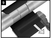
Remove the remaining release liner.
