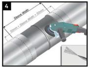
Ensure that the pipe is dry before cleaning. Using a power wire brush, abrade the pipe to a minimum of St3/SP3 (abrasive blast to Sa2.5/SP10 recommended). Lightly abrade the pipe coating adjacent to the cutback area to a distance of 50mm (2") beyond each end of the sleeve width.
