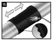
Shrinking has been completed when the adhesive begins to ooze at the sleeve edges all around the circumference. Finish shrinking the sleeve with long horizontal strokes over the entire surface to ensure a uniform bond.
