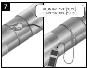
Pre-heat the joint area to the minimum required temperature. Using a temperature measuring device, ensure that the correct temperature is reached on the steel and at least 50mm (2") on each side of the sleeve.
