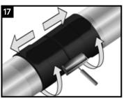
While the sleeve is still hot and soft, use a hand roller to gently roll the sleeve surface and push any trapped air up and out of the sleeve, as shown above. If necessary, reheat to roll out air.
