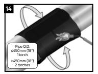
Using the appropriate torch, begin at the centre of the sleeve and heat circumferentially around the pipe. Use broad strokes. If utilizing two torches, operators should work on opposite sides of
