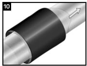
Completely remove the inner release liner from the sleeve and centre the sleeve over the area to be sealed.
