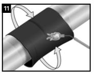
Using the appropriate sized torch, begin at the centre of the sleeve and heat circumferentially around the pipe. Use broad strokes.
