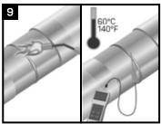
Pre-Heat the joint area to a minimum of 60°C (140°F). Using a temperature measuring device, ensure the correct temperature is reached on the steel and at least 50mm (2") on each side of the sleeve
