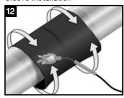
Continue heating from the centre toward one end of the sleeve until recovery is complete. In a similar manner, heat and shrink the remaining side. With a yellow backing, a pink-orange shade will appear when the proper temperature has been reached.
