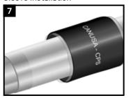
Ensure that there is no dirt or moisture inside the tube and that the tube is not cut. If the sleeve is not useable, a one-piece Wrapid Sleeve or Canusa Wrap sleeve should be used.
