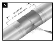
Ensure that the pipe dry before cleaning. Prepare the steel joint area to a minimum of St3 /SP3. Lightly abrade the pipe coating adjacent to the weld area to a distance of 50mm (2") beyond each end of the sleeve width.
