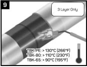
Pre-heat the joint area and abraded coating to the required temperature with the appropriate propane torch. If epoxy is applied, ensure that the epoxy is dry to the touch prior to sleeve installation. **Do not use an intense flame on the mainline coating**. If a film develops on the mainline coating because of preheat, use a surface abrasion tool to remove it.
