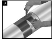
Apply mixed epoxy to a uniform specified thickness of 4-6 mils (100 - 150 microns) on all exposed bare metal using the applicator pads as supplied or an approved tool. Do not apply the epoxy to the mainline coating.
