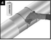
Ensure that the mainline coating edges are bevelled to 30°. If there is the presence of oil, grease, or other surface contaminants; clean the exposed steel and adjacent pipe coating with a solvent cleanser.
