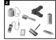
Canusa torch, propane tank, hose & regulator; Temperature measuring device, roller, knife; Appropriate surface abrasion device, solvent; Standard safety equipment (gloves, goggles, hard hat, etc.); Wet film thickness gauge Flame Intensity & Torch Size
