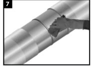
Wipe clean or air blast the steel and pipe coating to remove foreign contaminants.
