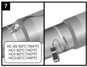
Pre-Heat the joint area to the minimum required temperature. Using a temperature measuring device, ensure that the correct temperature is reached on the steel and at least 50mm (2") on each side of the tape.
