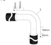
For other sizes, the following formula can be used: Length of tape =  $\pi$  x pipe diameter x L/W where L=length of area to be covered, and W= ½ of tape width (for 50% overlap)
