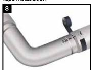
Starting at least 50mm (2") onto the pipe coating, begin wrapping the tape around the joint, ensuring a minimum 50% spiral overlap. Ensure that the adhesive side is placed onto the pipe. Remove any plastic release liners as the product is wrapped.
