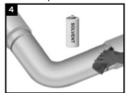
Ensure that the PE coating edges are beveled to 30°. Clean exposed steel and adjacent pipe coating with a solvent cleanser to remove the presence of oil, grease, and other contaminants.
