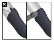
Warm the tape end and press down firmly. A hold-down tape can be used to secure the tape end.
