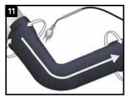
Using a torch, begin at the edge of the tape and heat circumferentially around the joint, working back to the other edge.
