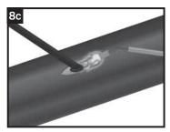
Heat the melt stick and the repair zone simultaneously with the torch and spread the melt stick over the damaged area. Keep the flame moving to prevent damage to the coating. Some ignition of the melt stick is acceptable.
