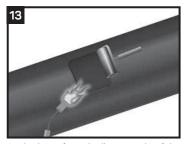
Apply the softened adhesive side of the patch to the damaged area and press down firmly. Heat the patch with a low intensity flame, and using a roller or a gloved hand, pat down and remove wrinkles. Roll to ensure a good bond.
