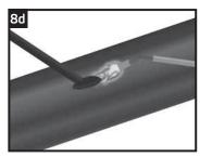
Continue spreading the melt stick over the repair zone until the entire area is covered. After sufficient melt stick material is on the surface, apply additional heat in quick back-and-forth strokes to create a smooth surface.
