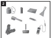
Propane tank, hose, torch & regulator; Appropriate tools for surface abrasion and cleaning, including wire brush, abrasive paper, rags & approved cleaner; Temperature measuring device. Misc. tools such as; knife, putty knife, roller, paint brush or paint roller, tape measure, and marker; Standard safety equipment; gloves, goggles, hard hat, etc.
