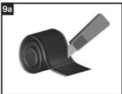
Fill deeper crevices with Canusa Mastic Filler (MF). Unroll the filler material and cut off the required amount, leaving the release paper in place.
