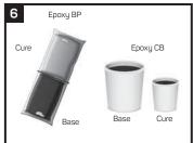
Follow the Preparation, Mixing and Application instructions provided with the supplied Canusa Epoxy Pack. For bulk quantities: mix the primer cure with the primer base (See Liquid Epoxy Product Data Sheet for Mixing Ratio). Stir for a minimum of 30 seconds to assure uniform mixture.
