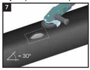
Using a hand grinder with a grit paper wheel, lightly abrade the repair area to expose FBE and/or bare metal surface and bevel the edges of the repair area to a 30° maximum angle. Using the hand grinder, lightly abrade the mainline coating in the major repair area. Continue to step 8.
