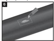
Using a knife, carefully cut out only the damaged coating into a smooth sided shape
