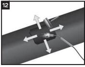
Using the roller and propane torch, continue heating and rolling from the middle to each edge. Continue until the adhesive is fully molten and has wet out on all edges.
