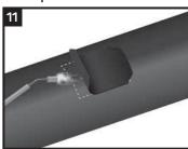
As the Repair Patch is laid on the pipe, place torch between Repair Patch Adhesive & pipe surface. Continue heating area as the Repair Patch is applied.
