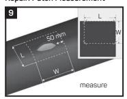
Measure the dimensions required for the Repair Patch. Cut the Repair Patch to the appropriate size to cover the patch area, with a minimum 50mm overlap from any point of the damage.
