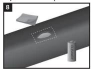
Using a grease and lint-free clean the prepared coating with an approved cleaner (i.e. xylol, xylene, trich, Isopropenol, Acetone, MEK, denatured alcohol) to remove the presence of oil, grease and other contaminants. For damages extending to steel, refer to the Polyethylene Repair Products Install Guide for application of liquid epoxy and filler material.
