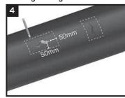
Using a marker, mark a rectangle 50mm beyond the damaged areas on all sides.
