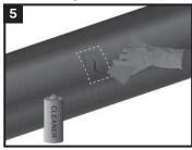
Using the sandpaper, abrade the mainline coating in the repair area. Remove all oxidation (shine) under area of the patch. Continue on step 8.
