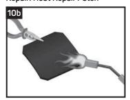
While holding the Repair Patch with a pair of pliers, use the propane torch to heat the black backing material until the Repair Patch becomes soft and flexible.
