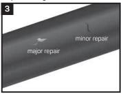
The type of repair is dependant on the extent of the damage to the mainline coating. If the damage to the coating (i.e. deflection, peeling, nick, etc.) results in a thickness of 50-80% of nominal, it is categorized as minor repair (see step 5). Major repairs (see step 6) are required when the coating thickness is less than 50% of nominal (i.e. tears, holes, destructive tests, blisters, etc.).
