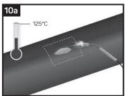
Using the propane torch, heat the repair area to 125°C. Using a digital thermometer, ensure the correct temperature has
