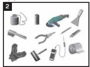
Propane tank, hose, torch & regulator; Appropriate tools for surface abrasion: grinder, 80-120 grit sandpaper; Appropriate tools for cleaning: rags & approved cleaner; Tools: roller, digital thermometer, knife, marker, measuring tape, scraper / spatula & pliers; Standard safety equipment; gloves, goggles, hard
