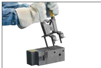
Fig. 6 Slide the handle clamp into the pre-drilled holes with the proper orientation for the thumbscrews.
