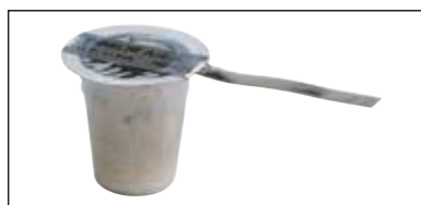
Fig. 8 Inspect the cup to ensure it is tightly sealed and the ignition strip is securely attached to the seal.
