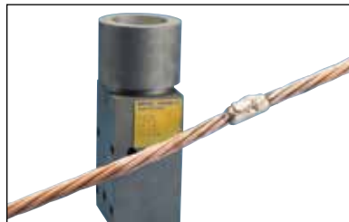
Fig. 31 Ready to make another Cadweld connection.
