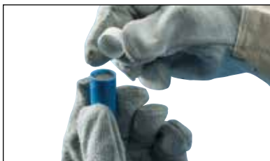
Fig. 10 Next, take the tube of welding material included in the Cadweld One Shot package and remove the lid over the crucible.
