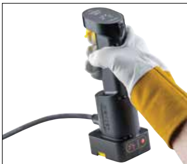
Fig. 13 Using the control unit, lift the trigger cover and press the ignition button and hold. You will see the 6 lights on the top of the control
