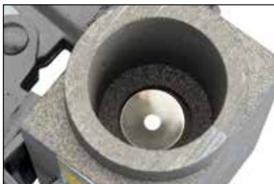
Fig. 19 Ensure that the steel disk is properly seated.
