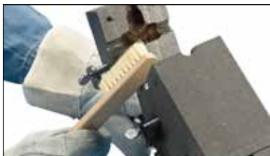
Fig. 24 Cadweld graphite molds will last for approximately 50 connections. Use a soft cotton cloth or a soft bristle brush (nVent ERICO part #T394) to clean inside the mold cavity and cover.
