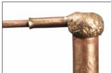
Fig. 16 You are ready to make another Cadweld connection.
