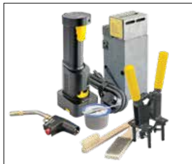
Fig. 2 Prepare the proper materials and equipment for the type of connection you are making. The Cadweld Plus system requires a graphite mold, mold clamp, Cadweld Plus welding material cup, natural bristle brush for mold cleaning, wire brush for cleaning/preparing conductors, control unit, and propane torch.
