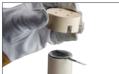
Fig. 10 Place the ceramic lid onto the mold.
