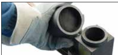
Fig. 27 Remove the alligator clips from the igniter pin. Remove the graphite cover of the Cadweld Exolon mold.
