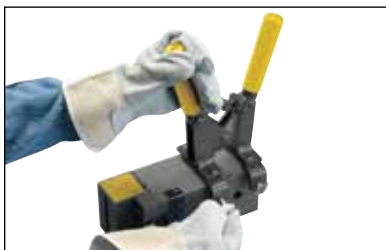
Fig. 7 Tighten the clamp thumbscrews onto the mold.
