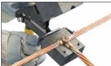
Fig. 25 Open the mold and remove the connection. Use care to prevent chipping the mold. Avoid contact with hot materials. See the “nVent ERICO Cadweld Quality Standards” section to see whether a quality connection has been made.
