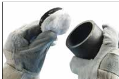
Fig. 14 Each Exolon package contains 2 filters for a low emission connection. Insert the white ceramic and black graphite filters into the mold cover. (Filters must be changed every 4 connections.)
