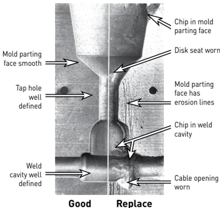
A ERICO CADWELD mold is designed to last for an average of 50 connections. This will vary according to the care given the mold during use.
