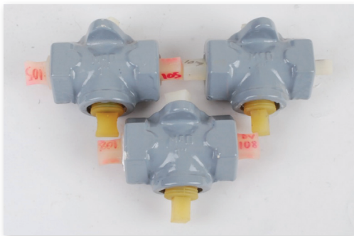
The test samples above are shown following 3,000 hours of salt spray exposure. These are zinc coated castings with two coats of paint.
