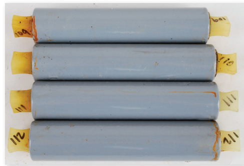
The test samples above are shown following 3,000 hours of salt spray exposure. These are steel pipe with two coats of paint.
