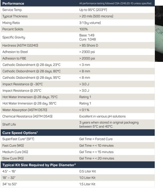
1 Gel times were measured @ 23°C (73°F). For more information please refer to Canusa's Technical Bulletin – High Build Epoxy Cure Profiles. 2 SuperFast Technology (SFT) is used as repair material in FBE coating plants.
