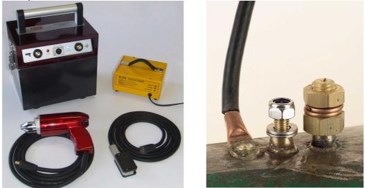
The brazing process is controlled by means of the fuse wire on the brazing pin. The capacity is approximately 15 brazes with the standard type of brazing pin per battery charge but it can easily be increased by a battery charger mounted in a vehicle, the batteries being charged up during transportation between workplaces. When alternating between charging and brazing it is possible to increase the capacity up to 5 times during a working day.
